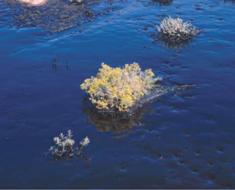
Crude oil with very low produced water content (waste oil and tank bottoms look very similar)
