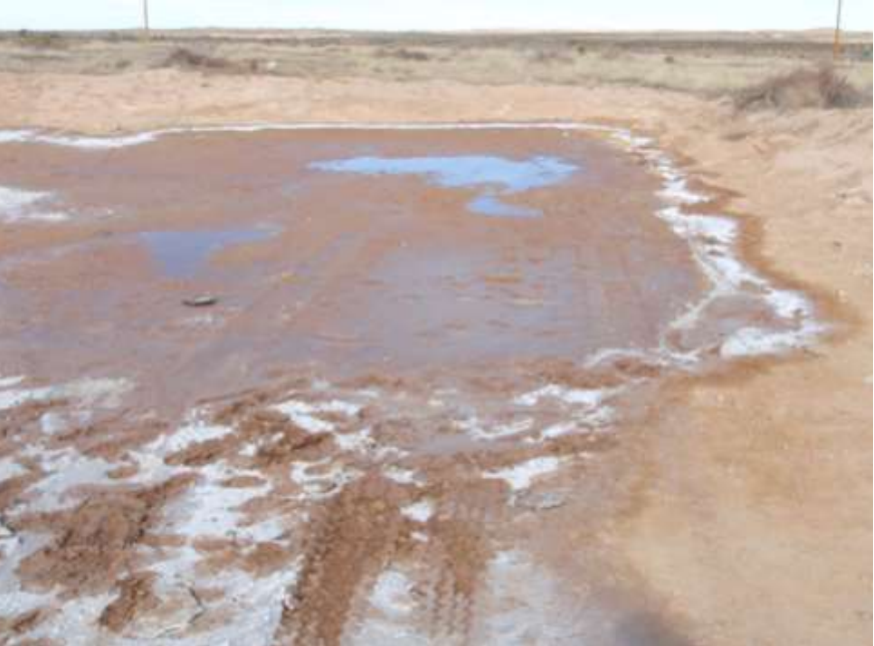
Brine range produced water with trace oil (dumped within 24 hours; gypsum soil)
