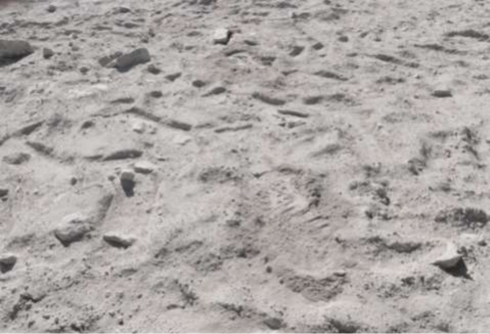
Bulk bentonite clay mix for making up drilling fluids (bulk dry cement looks very similar)
