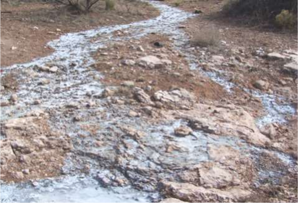
Brine cement truck rinsate (watery and thin as pictured) or brine cement (thick and clumpy)
