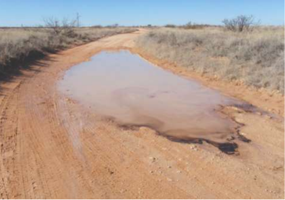
Brine range produced water with skim oil (several hours old, salts just beginning to pop out on left side)
